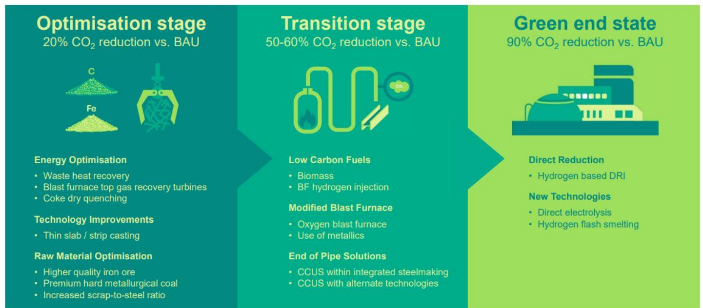
Figure 17: BHP's 3-stage steel decarbonization framework
